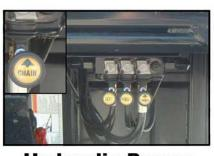
Hydraulic Power The Power Bed is powered from the existing hydraulic system installed on the truck to run the conveyor. A simple forward and reverse hydraulic valve is all that is needed to operate the Power Bed.
